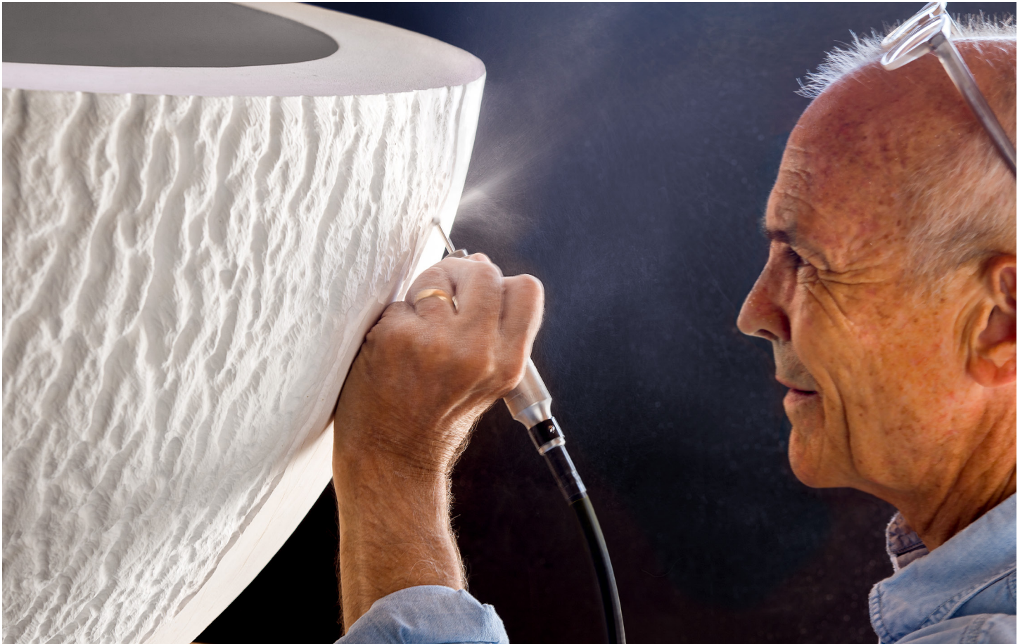
Above: Carving the Nutshell series by hand was no small feat. In a process that took nearly two months of work, Kornegay etched a pattern in the surface of a blank container that would later be used to make a master mold.
